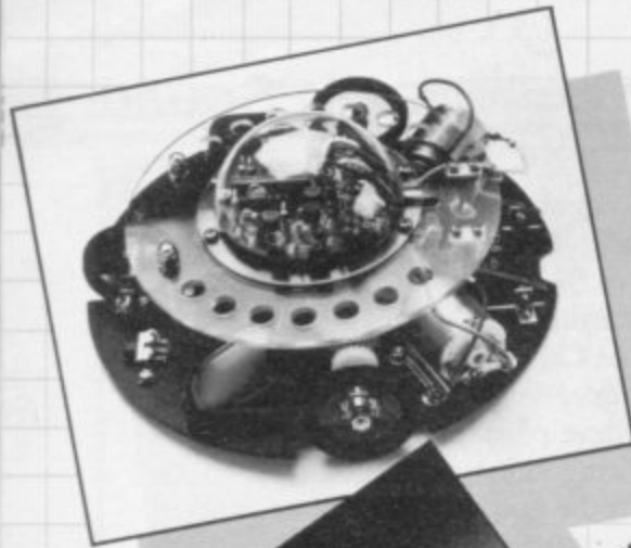
Line Tracer II £17.99 Draw a line and the infra-red sensor picks it up and sends this 3 wheeled, twin motored robot along the course you plot.
